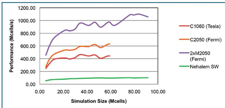
throughput, ECC support, and improved overall performance. In addition, two of these cards can be connected in parallel to allow higher performance and larger domain sizes. The Series 20 shows remarkable improvement over the Series 10 (Tesla) in the above plot, but it positively eclipses the solver speed of the Nehalem software solver. Solving this particular problem in CPU-based software mode simply becomes too onerous to be practical.
